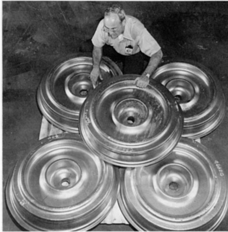
Fig. 4 Forged Ti-6Al-4V jet engine fan disks are 890 mm (35 in.) in diameter and weigh 249 kg (548 lb). Courtesy of Wyman-Gordon Company
