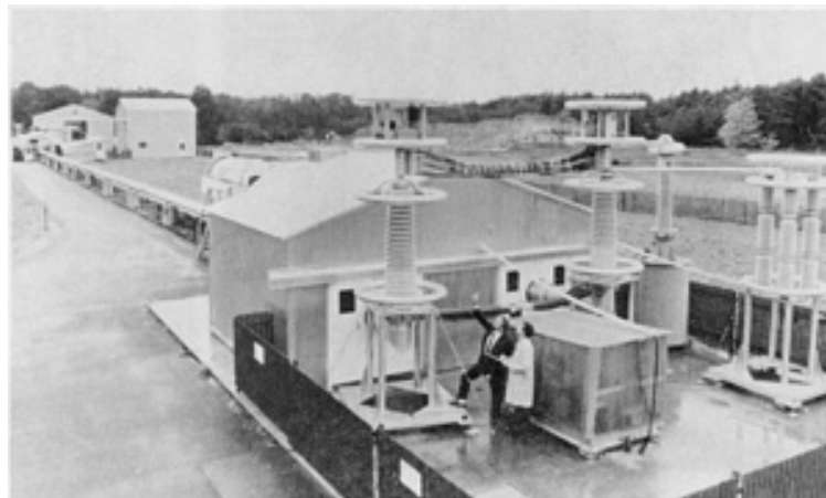
Fig. 30 The 100 m (330 ft) experimental test station at Brookhaven National Laboratory for power transmission
