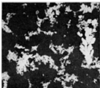
Fig. 6 Electrolytic copper powder showing dendritic structure. 85×
