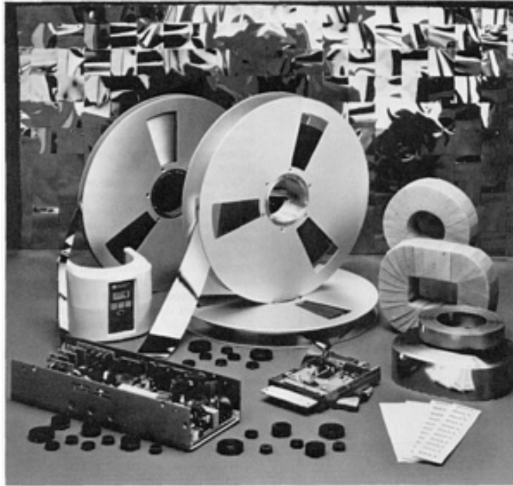
Fig. 18 Various parts that use metallic glasses. Most prominently featured are two spools of as-cast amorphous alloy for high-frequency and antitheft applications. Also shown (right side) are four wound magnetic cores made from amorphous alloy ribbon. Several high-frequency epoxy-encapsulated small cores are shown in the foreground. Such cores are used in switch-mode power supplies, magnetic amplifiers, chokes, and other electronic devices to be incorporated in electronic assemblies such as the one shown. At the lower right are bar code markers containing a strip of metallic glass. In the background is a woven blanket of metallic glass used in magnetic shielding. Courtesy of H.H. Liebermann, Allied-Signal Inc.
