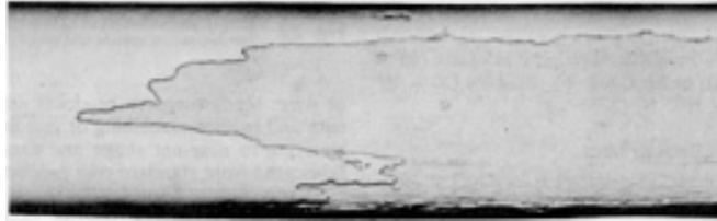
Fig. 24 Recrystallized microstructure of doped tungsten wire
