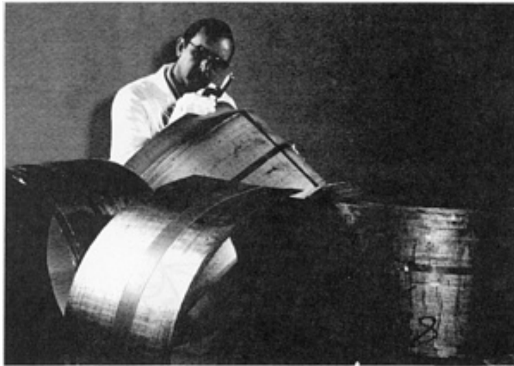
Fig. 11 Direct cast sheets of IC-50 (Ni-23.5Al-0.5Zr-0.08B, at.%) and IC-218 (Ni-16.7Al-8.0Cr-0.4Zr-0.08B, at.%) Ni 3 Al alloys. Source: Ref 84
