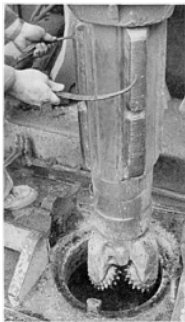
Fig. 48 Rotary blast-hole tricone bit with embedded carbides and fitted with carbide stabilizer bars
