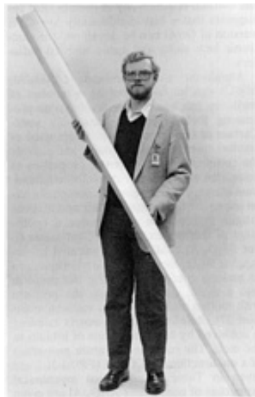
Fig. 4 Advanced aircraft stabilator spar made from an SCS/Al MMC. Courtesy of Textron Specialty Materials
