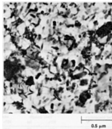
Fig. 7 TEM micrograph of an RS-P/M Al-8Fe-4Ce alloy showing fine Al-Fe-Ce phases that strengthen the 1 mm (0.040 in.) thick sheet. Courtesy of G.J. Hildeman and L. Angers, Alcoa Laboratories
