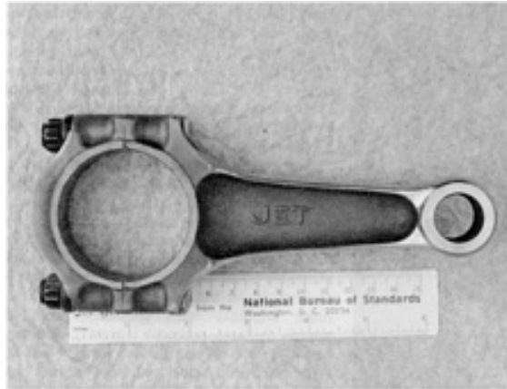
Fig. 6 Forged alloy connecting rod for a racing engine is indicative of increasing automotive applications for titanium. Component, courtesy of Jet Engineering Inc.; photograph by R.T. Kieपुरa, ASM INTERNATIONAL
