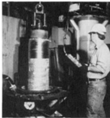
Fig. 1 Consumable NbTi electrode being prepared for its final vacuum-arc remelt. Courtesy of Teledyne Wah Chang Albany
