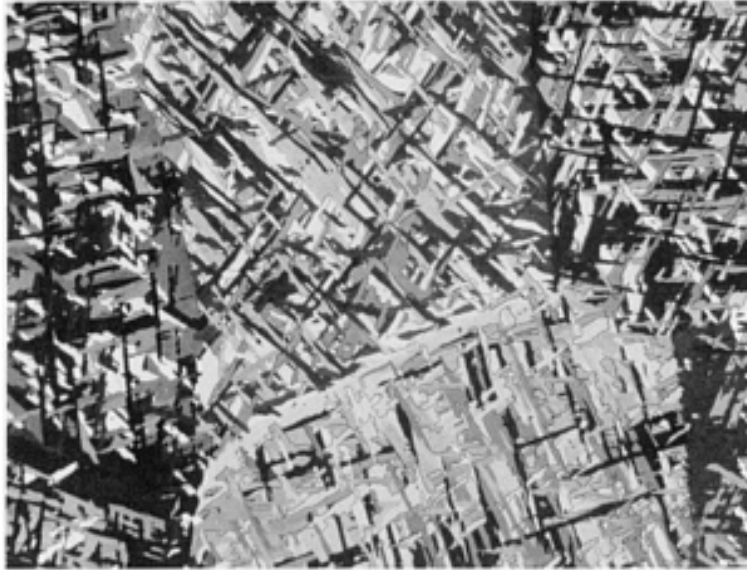
Fig. 3 Zirconium cooled from 950 °C (1740 °F). Cooling transformation resulted in a Widmanstätten structure. 75×
