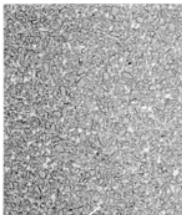
Fig. 25 Microstructure (at 1500 \times ) of a typical spinodal titanium carbonitride cermet. The manufacturing process, called spinodal decomposition, minimizes grain growth and consistently produces nonporous material. Courtesy of Teledyne-Firth-Sterling
