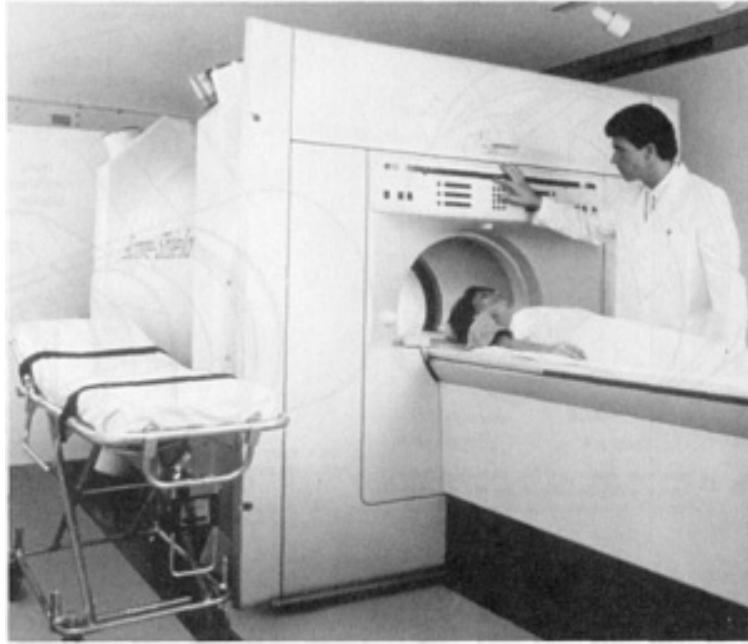
Fig. 30 Whole-body 2 T (20 kG) MRI unit with an active shield. Courtesy of Oxford Superconducting Technology
