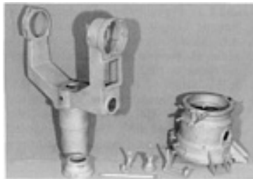
Fig. 17 Titanium housings for aerospace optical applications produced by the investment casting process.
