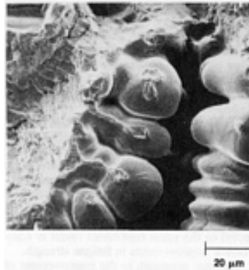
Fig. 6 Dendritic structure present in the surface shrinkage porosity of an as-cast Ti-6Al-4V component
